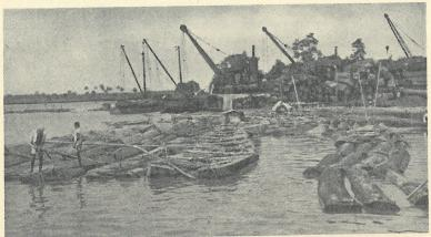
A raft of logs arriving at a saw mill. Two of the raft men's huts can be seen in the middle distance. The cranes are used to lift the logs out of the water and pile them up in the store.
