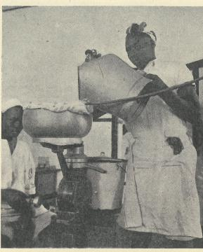
Pouring milk into a cream separator machine that whirls round at a high speed and separates the watery portion from the cream. The cream is used for butter-making; the watery portion (the separated milk) is a valuable food for pigs.
