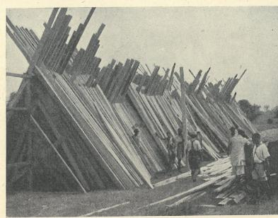
Timber must be carefully seasoned after sawing. Before it is stacked in the seasoning sheds it is exposed for several days in the open.
