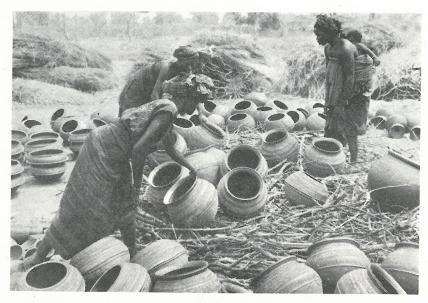
Potters on Jebba Island preparing to build up a pile of sun-dried pots preparatory to firing. The fuel used consists of small branches and dried grass.
