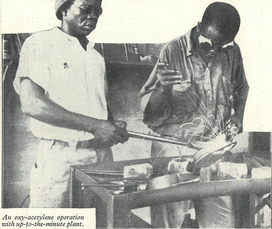
*An oxy-acetylene operation with up-to-the-minute plant.*
